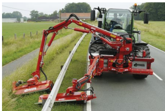
MK mower combination consisting of DUA 700 and RSM for mowing behind and under guide rails
