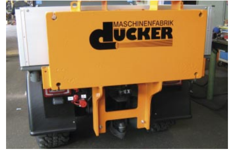
Counterweight in the mounting brackets of narrow-gauge vehicles
