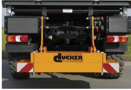
Counterweight in the Unimog's mounting brackets
