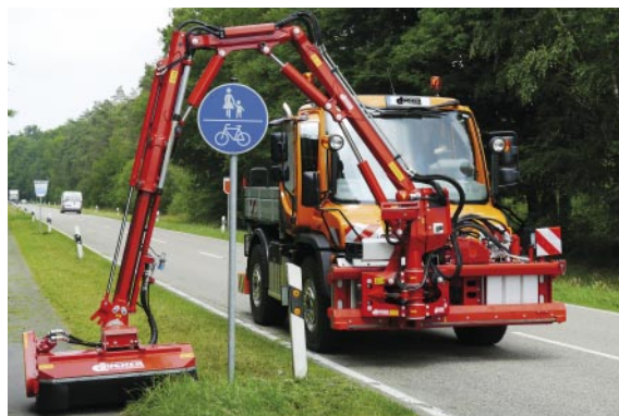
DUA 800 – The telescopic arm makes it possible to drive over
