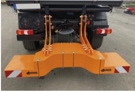
Counterweight (spreader version) in the Unimog mounting brackets
