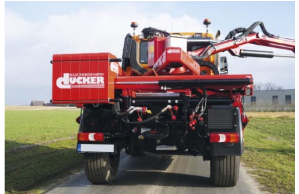
The hydraulically adjustable counterweight
