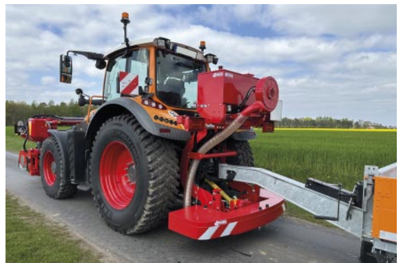
With the DÜCKER hydraulic unit, the rear trailer coupling remains freely accessible.
