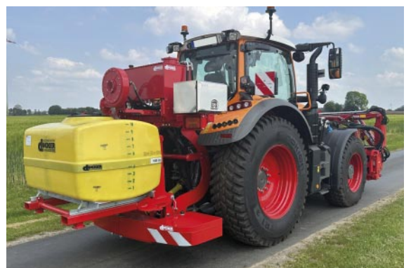
Water tank, mounted in the coupling points of the hydraulic unit.
