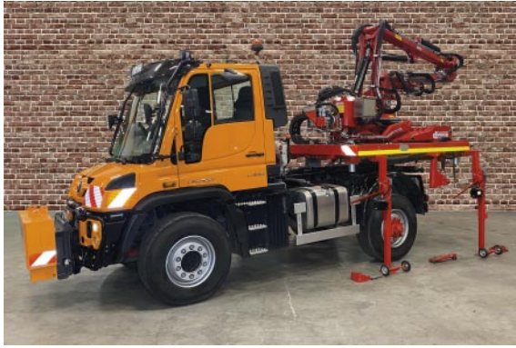
Easy removal of base frame and stabiliser
