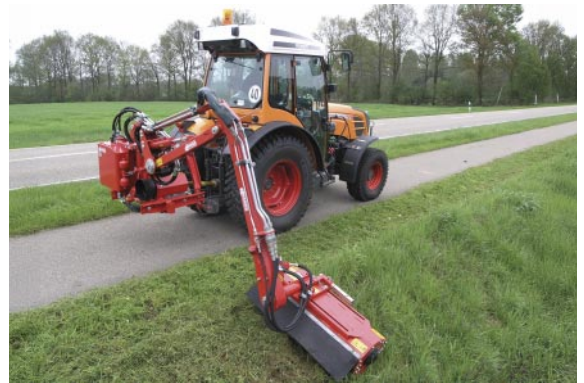
KBM 350 in rear mounting with flail mower head
