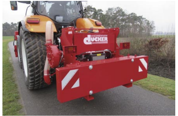
Hydraulic unit with positioning of the counterweight behind the unit
