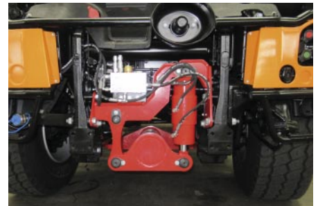
Hydraulic torsion frame on the Unimog
