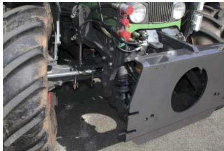
Vehicle plate with hydraulic axle support
