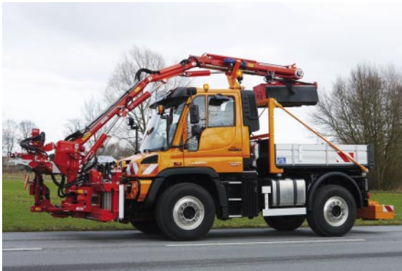
MK 25 in rear transport position with parking frame
