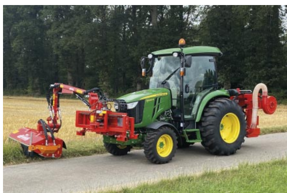
UNA 200 in split design, hydraulic unit at the
