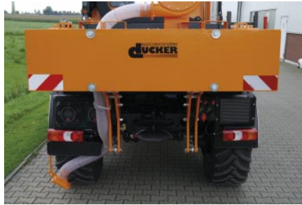
Counterweight in the Unimog's mounting brackets (moved upwards)
