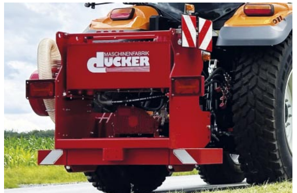
Hydraulic unit with positioning of the counterweight under the unit
